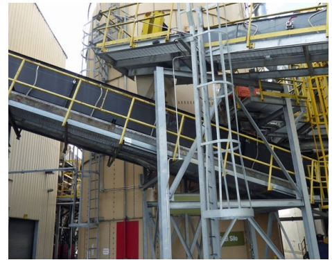
Laidig Model 543-26' Cantilever Reclaim System and one (1) steel bolted silo. Size 26.2 ft dia X 72.5 ft tall
